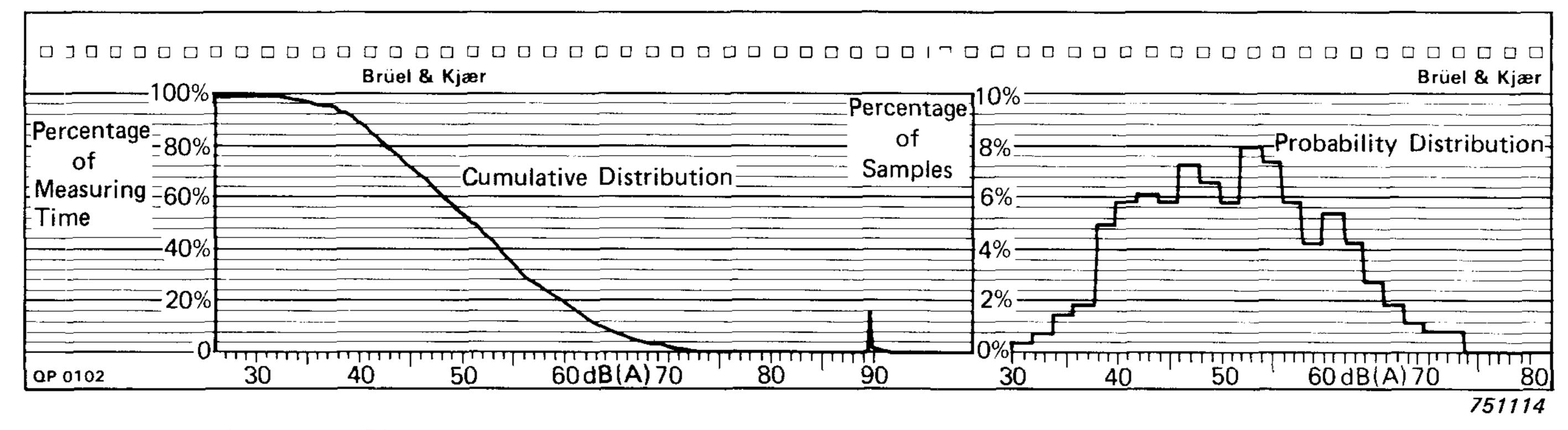
Recording of Cumulative Distribution curve and Probability Distribution histogram made on the portable Level Recorder Type 2306
