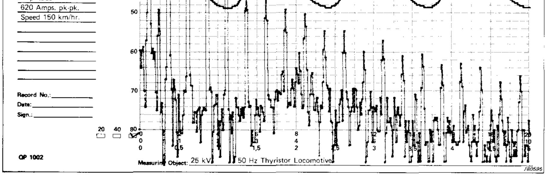
Although the primary current waveforms in these two figures are very similar, the dip in the 11th harmonic in the upper trace indicates that the second bridge had not quite reached full conduction (i.e., phase-advance). The lower figure shows full full conduction on both bridges, i.e., diode operation of the locomotive
