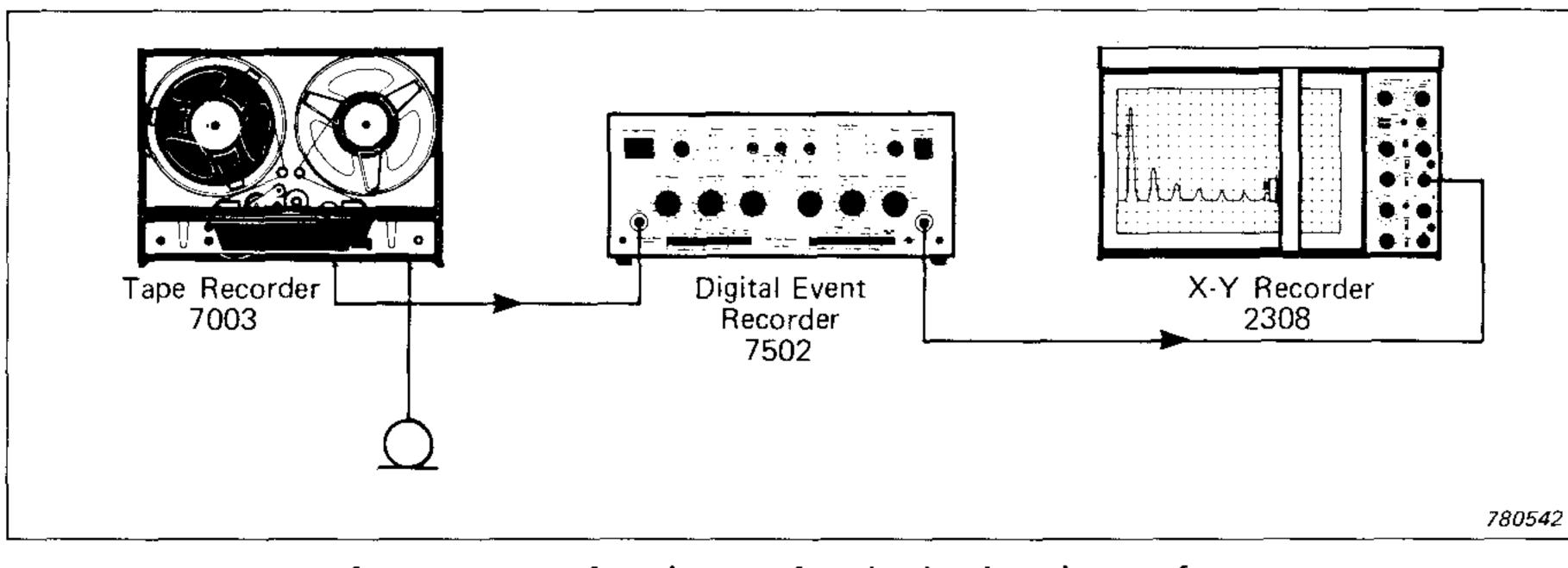
Arrangement of equipment for plotting inrush waveforms
