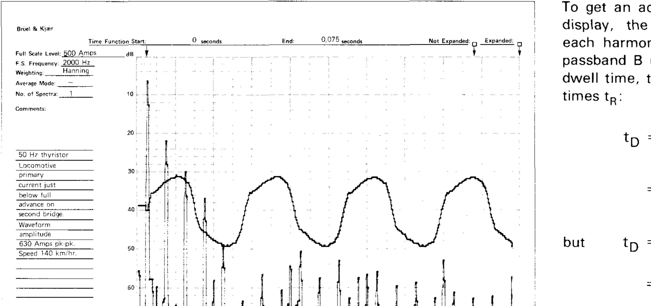
To get an accurate and undisplaced display, the total time for which each harmonic lies within the 3 dB passband B (which is known as the dwell time,  $t_D$ ) should be about four times  $t_R$ :
