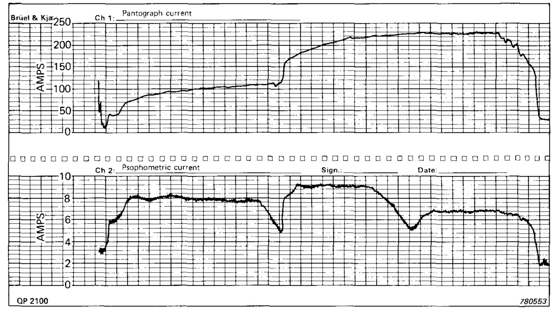
Log of pantograph current (= primary current) and psophometric current as functions of time, during an acceleration at constant armature current. The time scale is 5 s/div. For the first 80 s only one bridge is conducting
