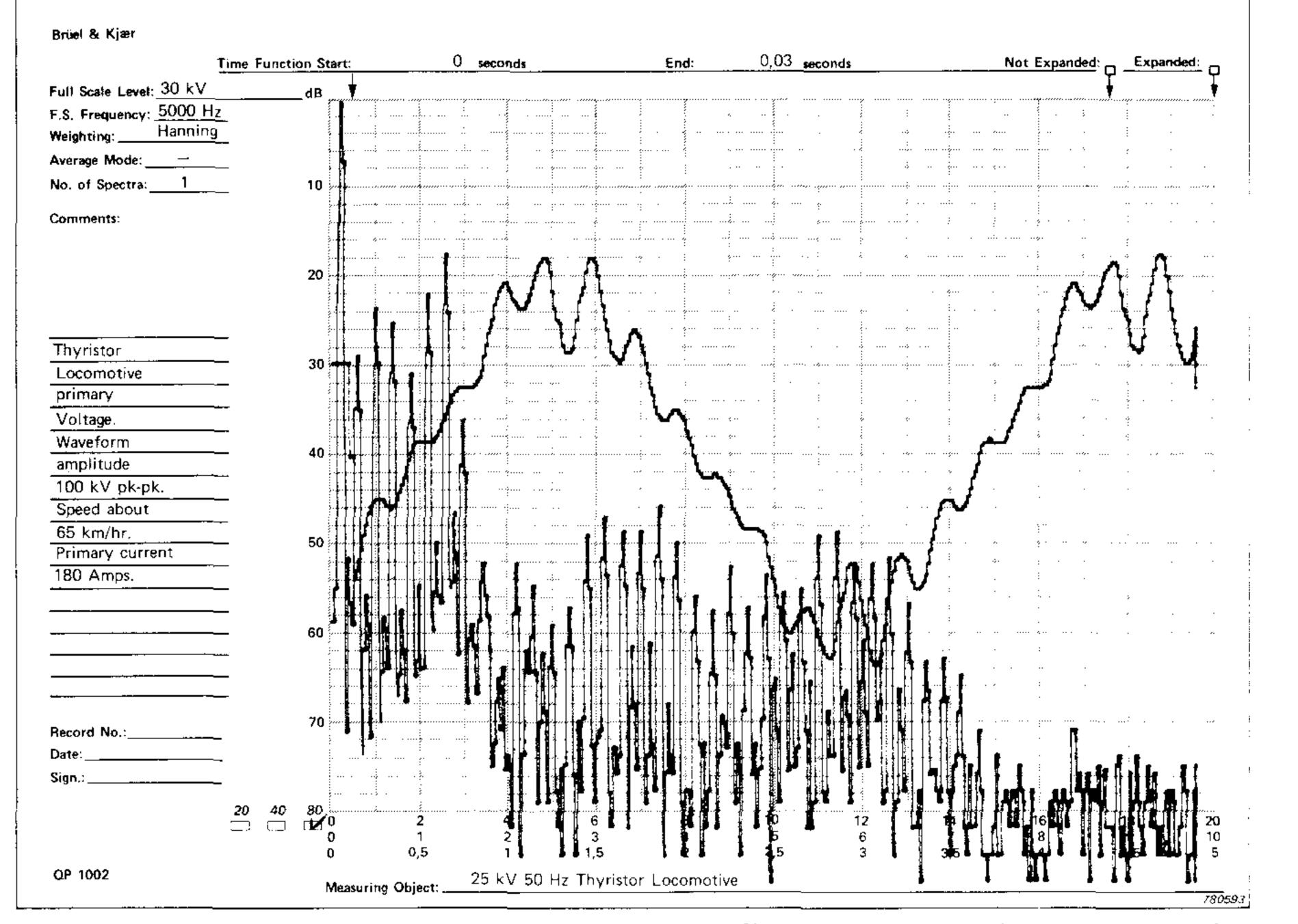
$n_{max} = 7$ , seconds, which is 350 Hz. Although a locomotive might accelerate as slowly as this, an EMU would normally advance from 0° to 180° on one rectifier bridge much more quickly, so the number of harmonics which may be usefully observed with a swept-frequency analyzer is very restrictive.
