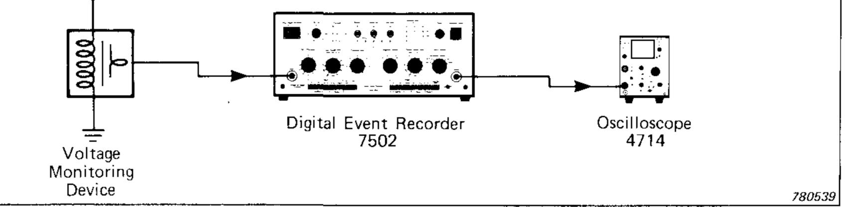
Arrangement of equipment for capturing and measuring line voltage surges
