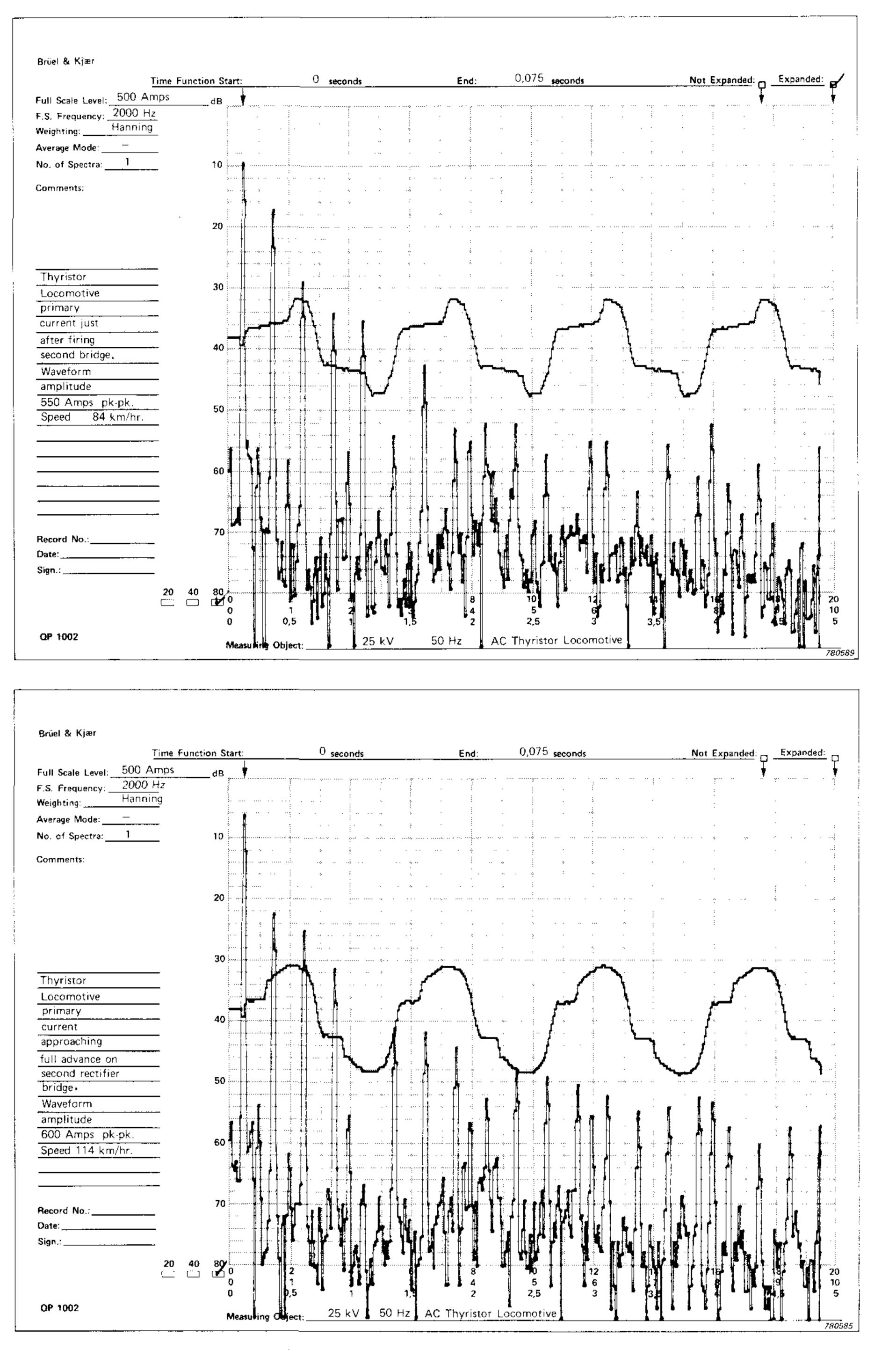
The filter bandwidth B should be narrow enough to resolve adjacent harmonics differing in amplitude by more than 10 dB. This means that B should be about one-third of the interval between peaks. If it is required to resolve only odd harmonics (which is all an ideal assymmetric half-controlled bridge rectifier generates in the supply),
