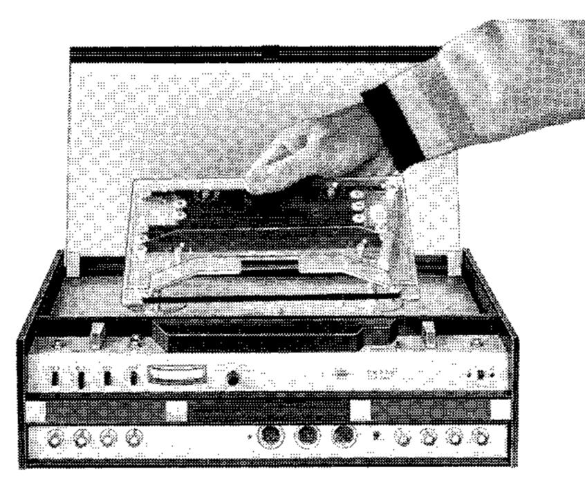
Illustration showing the use of a tape-loop cassette with the Type 7003 Tape Recorder
