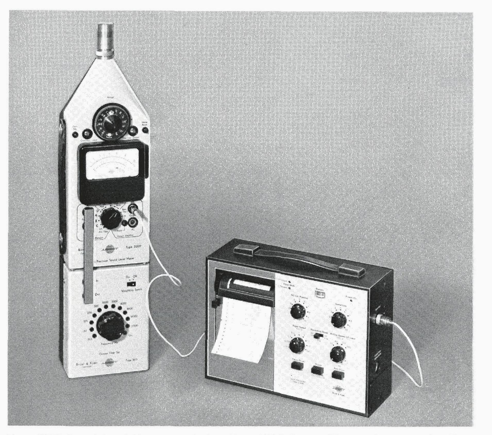
Measuring the vibration modes of the magnetic cores which generate most of the sound is not as difficult as it might appear, particularly if a sound level meter is already available. All that is needed then is an accelerometer.
