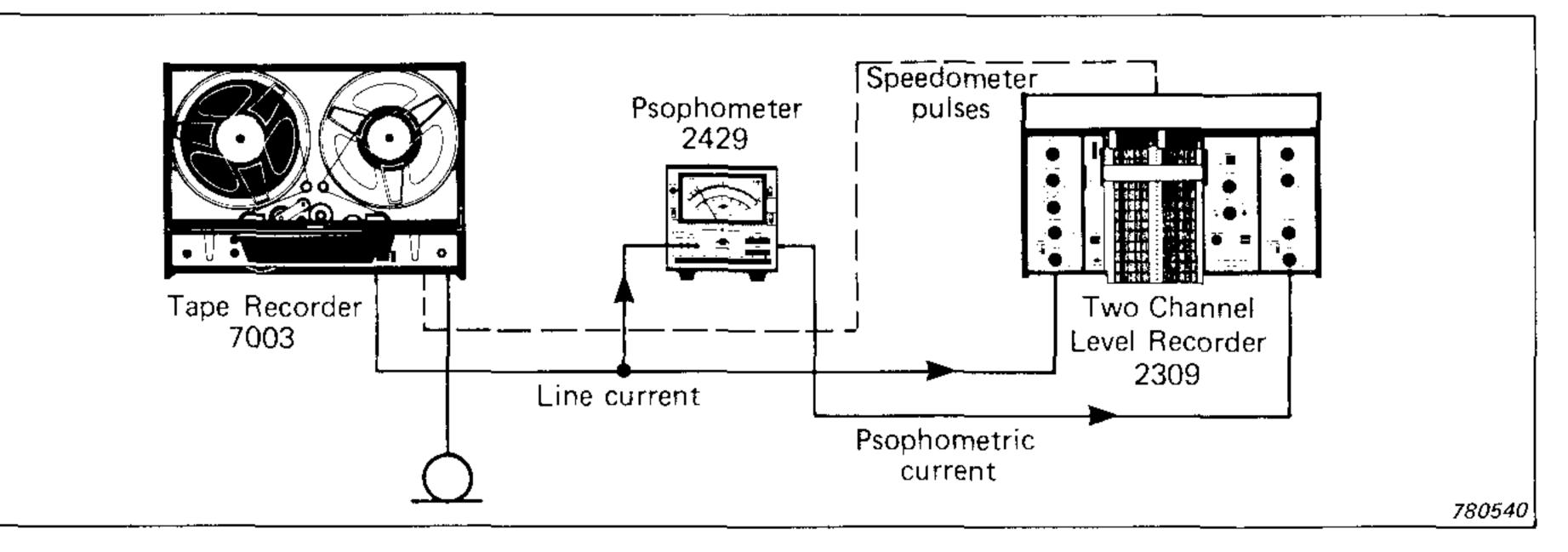
differential characteristic, it is quite possible to measure it on an existing system, and so predict the level of induced psophometric noise from new electric traction unit by measuring the psophometric current injected into the supply by the new equipment.
