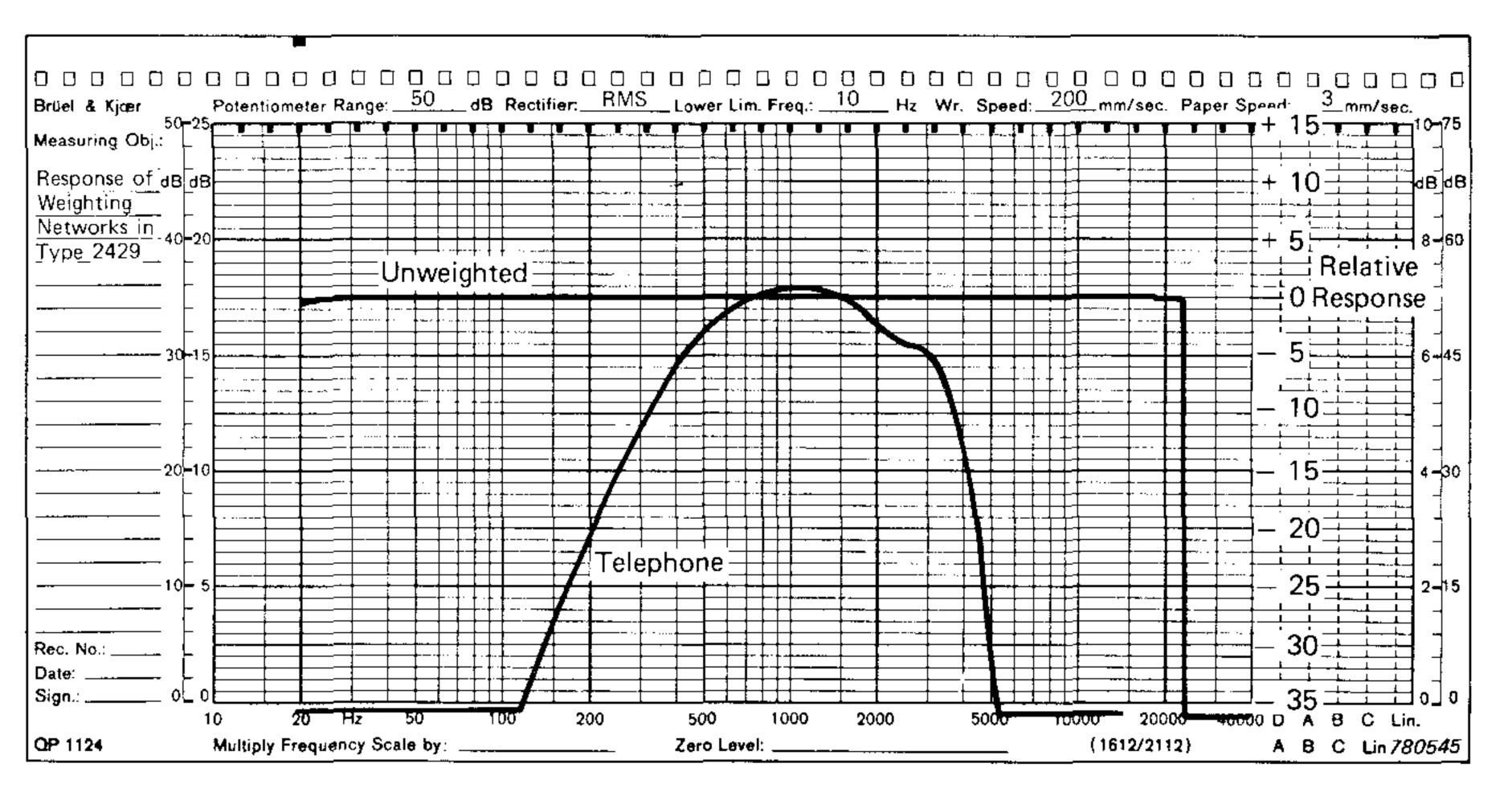
cording to the results of statistical experiments on human subjects. The weighting filter used for this purpose is known as a psophometric filter, and the complete instrument is a psophometer. It is also common to refer to the noise mea-
