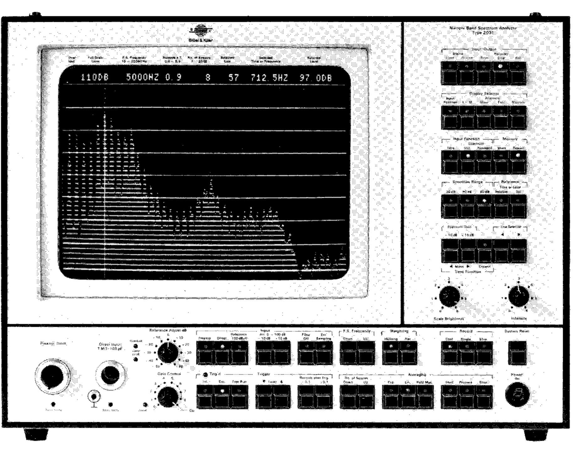
Type 2031 Real-Time Narrow-Band Frequency Analyzer
