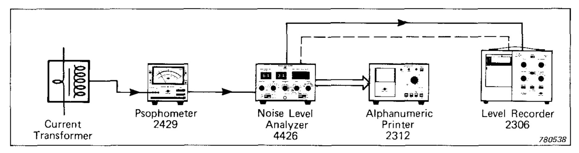
rent in the case of AC EMU's. A good way to obtain or supply that evidence is to connect up a Type 2429 Psophometer, a Type 4426 Noise Level Analyzer and a Type 2312 Alphanumeric Printer.
