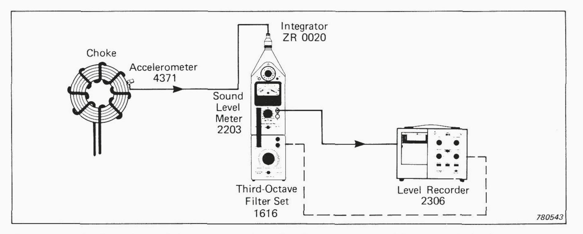
In the chopper application the accelerometer would be attached by a magnet or wax to different parts of the choke core, in different orientations, and the output connected via the cable provided, and an integrator Type ZR 0020 (to measure displacement or velocity) to the microphone socket of the sound level meter. The latter could then be used to measure the level of vibration, and its AC output fed to an oscilloscope
